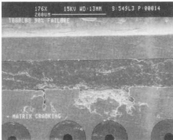
Figure 4. SEM photo of (0/90)<sub>S</sub> specimen at 90% of failure load showing matrix cracking.
