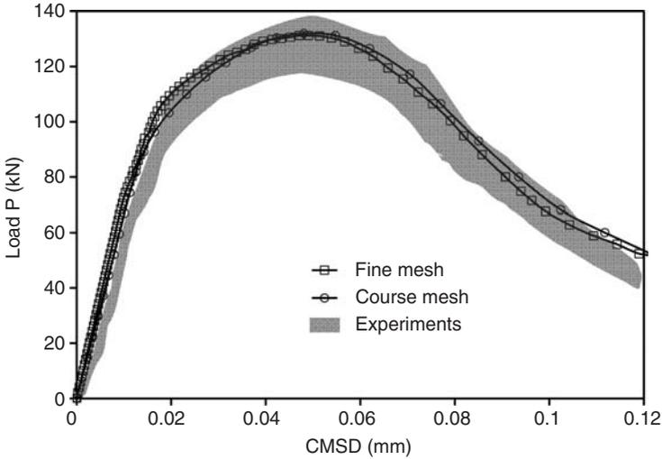
**Figure 9.** Comparison of the load vs CMSD for mesh refinement of the four-point bending notched beam. Experimental data by Arrea and Ingraffea (1981).
