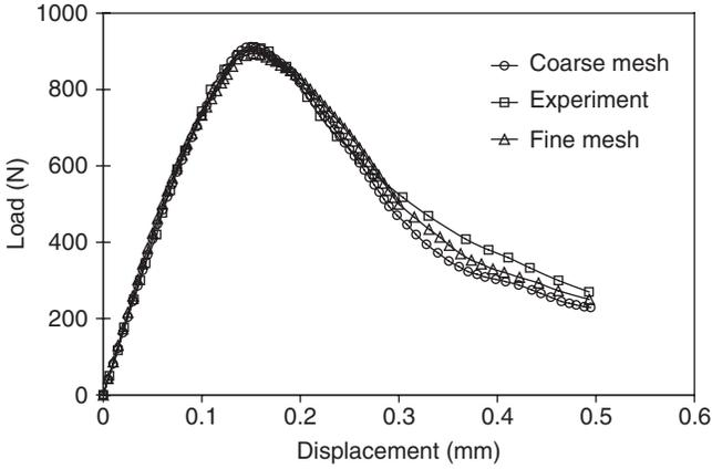
**Figure 6.** Comparison of the load vs displacement for mesh refinement of the three-point bending notched beam. Experimental data by Malvar and Warren (1988).
