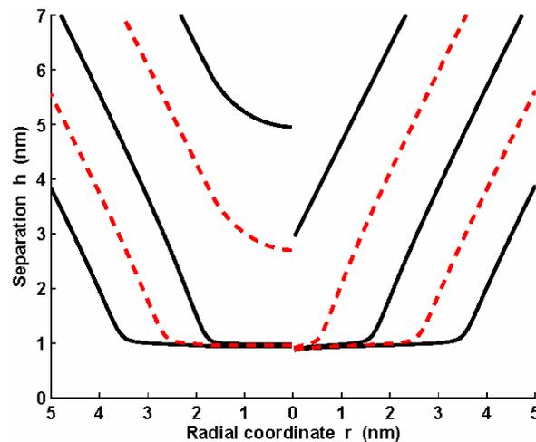
**Figure 4** Separation  $h(r)$  due to the Lennard-Jones adhesive law at positions  $h_0^* = 3, 1, -1, -3, -5$  nm for loading (right) and unloading (left), for the round-tipped with tip radius  $r_i = 4$  nm (see online version for colours)
