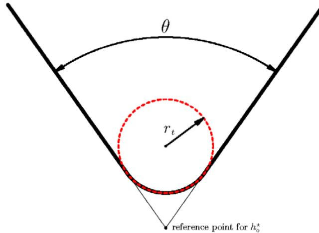
Simulations were conducted for  $r_t = 0$  (a sharp-tipped cone) and  $r = 1, 2, 4,$  and  $6$  nm, with  $\theta = 60^\circ$  in all cases. (AFM tips with tip end radii at least as small as 2 nm are readily commercially available). The position  $h_0^*$  is defined as the distance between the tip and the sample at  $r = 0$  if the tip was a sharp-tipped cone, and it varies from 5 nm to  $-5$  nm in 0.05 nm steps.
