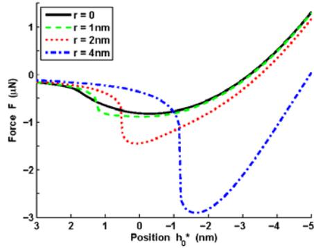
**Figure 6** Total force  $F$  vs. position  $h_0^*$  for loading for all indenter shapes, for the Poisson-Boltzmann repulsion surface force law (see online version for colours)
