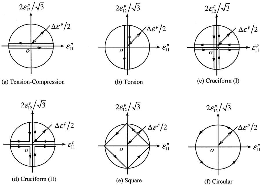
Fig. 7. Cyclic plastic strain paths with  $\Delta\epsilon^p/2=0.2\%$  and a constant plastic strain rate  $\dot{p} = 3 \times 10^{-5}/s$  (Tanaka et al., 1985).
