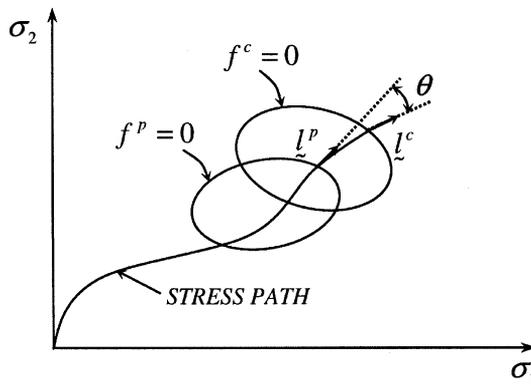
Fig. 6. Schematic representation of the nonproportionality measure ( $\theta$ ).
