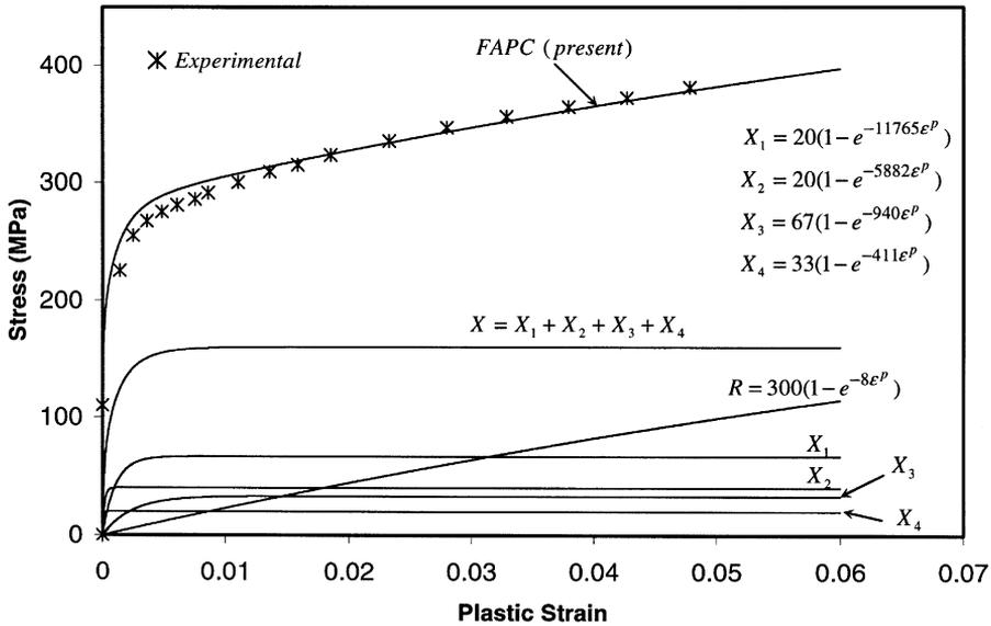
Fig. 3. Superposition of several kinematic hardening models under uniaxial tensile loading for 316L stainless steel ( $M=4$ ).
