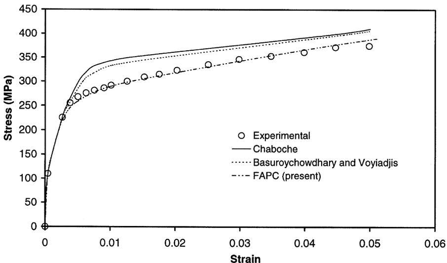
Fig. 4. Finite Element Simulations of uniaxial tensile loading for 316L stainless steel.
