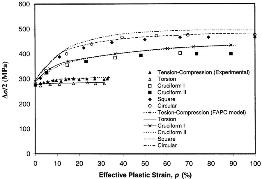
Fig. 8. Effect of cyclic plastic strain paths on cyclic hardening of 316 stainless steel ( $\Delta\epsilon^p/2=0.2\%$ ,  $\dot{p}=3 \times 10^{-5}/s$ ).
