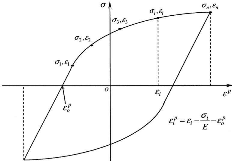
Fig. 2. Stabilized full-cycle of symmetrical uniaxial tensile stress-strain data representing the hardening in the nonlinear kinematic hardening model.
