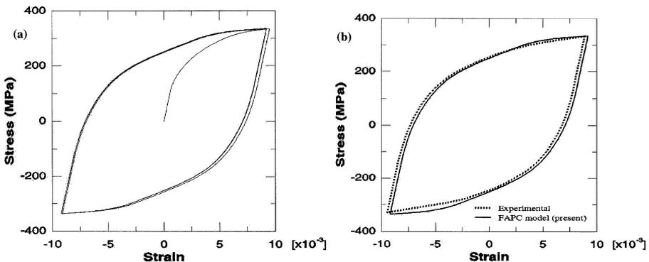
Fig. 5. Cyclic hardening under uniaxial stress-controlled cyclic loading of 316L stainless steel at room temperature: (a) numerical simulation, (b) identification of the stabilized cycle.
