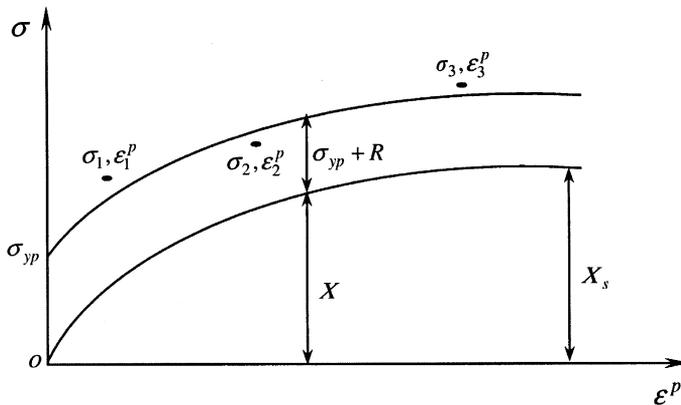
Fig. 1. Half cycle of stress-strain data representing the hardening in the nonlinear kinematic model (● represents experimental data at three different stress levels).
