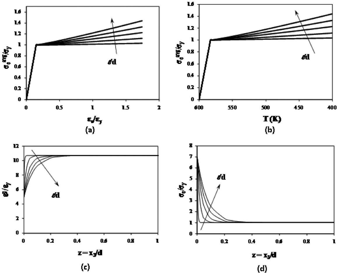
Fig. 3 Thermal cooling of an aluminum-silicon thin film-substrate system by 200 K due to interfacial hardening only ( $\delta_1=0$  and  $\delta_2=50$ ). Different film thicknesses are represented by  $\ell/d=0.1, 0.5, 1, 1.5,$  and  $2$  for: (a) average stress versus strain, (b) average stress and temperature, (c) plastic strain through the thickness, and (d) stress through the thickness.
