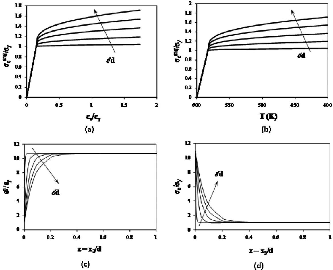
Fig. 4 Thermal cooling of an aluminum-silicon thin film-substrate system by 200 K due to both interfacial yield strength and hardening ( $\delta_1 = \delta_2 = 0.5$ ). Different film thicknesses are represented by  $\ell/d = 0.1, 0.5, 1, 1.5,$  and  $2$  for: (a) average stress versus strain, (b) average stress and temperature, (c) plastic strain through the thickness, and (d) stress through the thickness.
