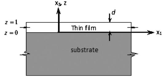
Fig. 1 An elastoplastic thin film of thickness  $d$  on an elastic substrate
