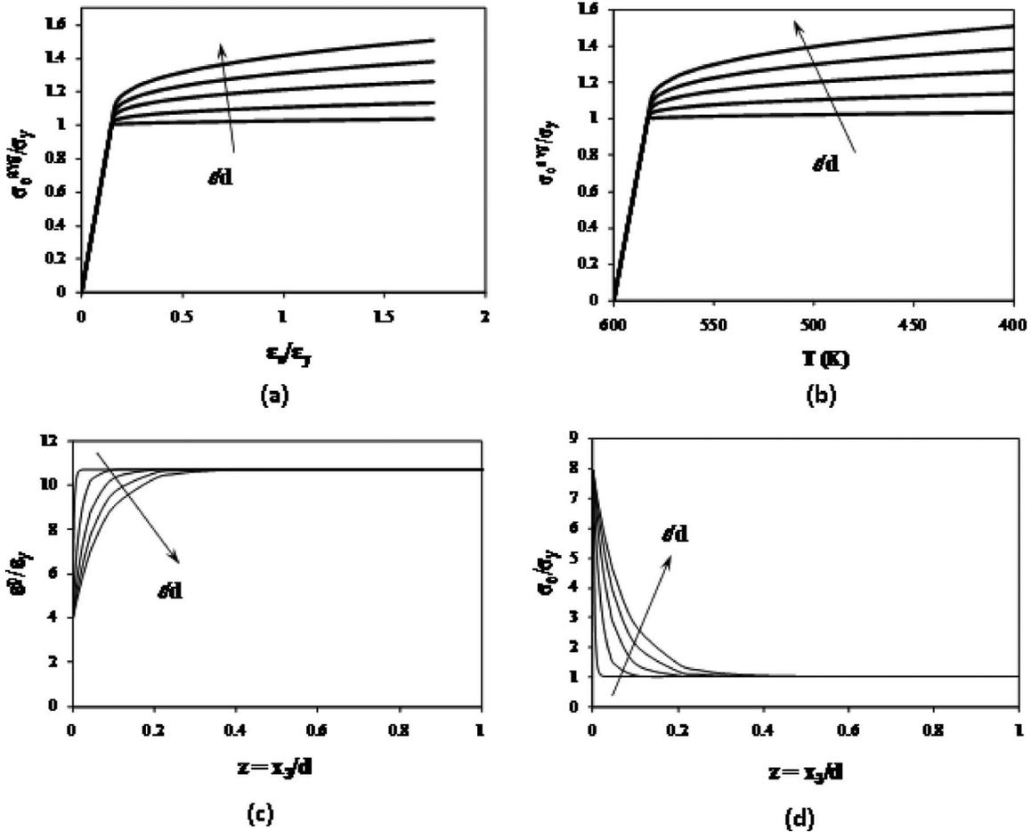
Fig. 2 Thermal cooling of an aluminum-silicon thin film-substrate system by 200 K due to interfacial yield strength only ( $\delta_1=0.35$  and  $\delta_2=0$ ). Different film thicknesses are represented by  $\ell/d=0.1, 0.5, 1, 1.5,$  and  $2$  for: (a) average stress versus strain, (b) average stress and temperature, (c) plastic strain through the thickness, and (d) stress through the thickness.
