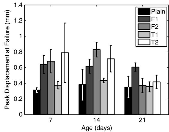
**Fig. 4.** Effect of the CNFs and MWCNTs on the strain capacity of cement paste
