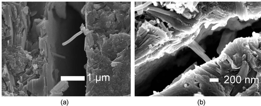
**Fig. 13.** (a) SEM image of a microcrack bridged by a CNF; (b) CNF pulled out from a microcrack
