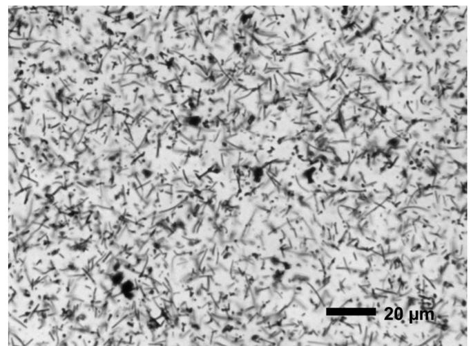
**Fig. 2.** Effect of ultrasonic mixing on the dispersion of CNFs in an aqueous solution containing a surfactant and sonicated for 15 minutes
