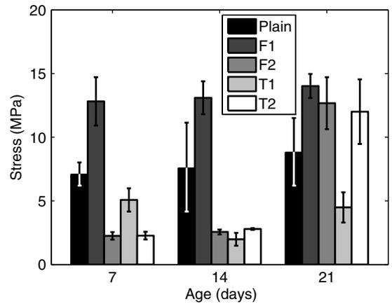
**Fig. 5.** Effect of the CNFs and MWCNTs on the ultimate strength of cement paste
