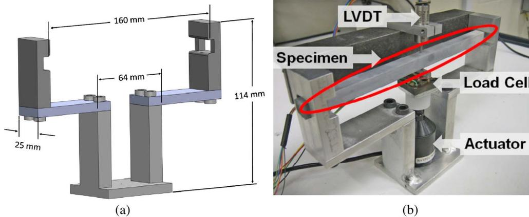
**Fig. 1.** (a) 3D model of flexural load frame model; (b) test frame setup for three-point bend with cement specimen in place (Image by Bryan Tyson)
