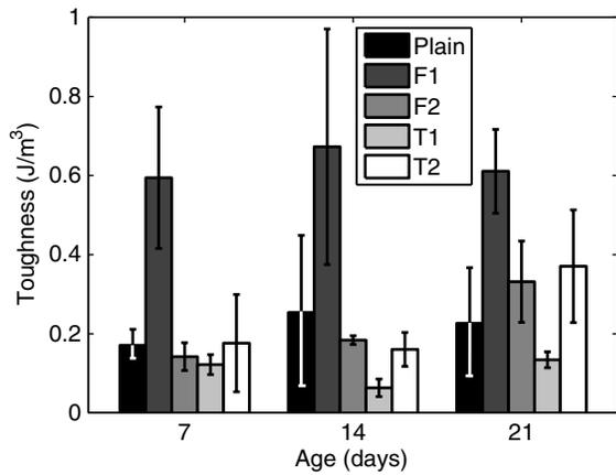
**Fig. 7.** Effect of the CNFs and MWCNTs on the fracture toughness of cement paste
