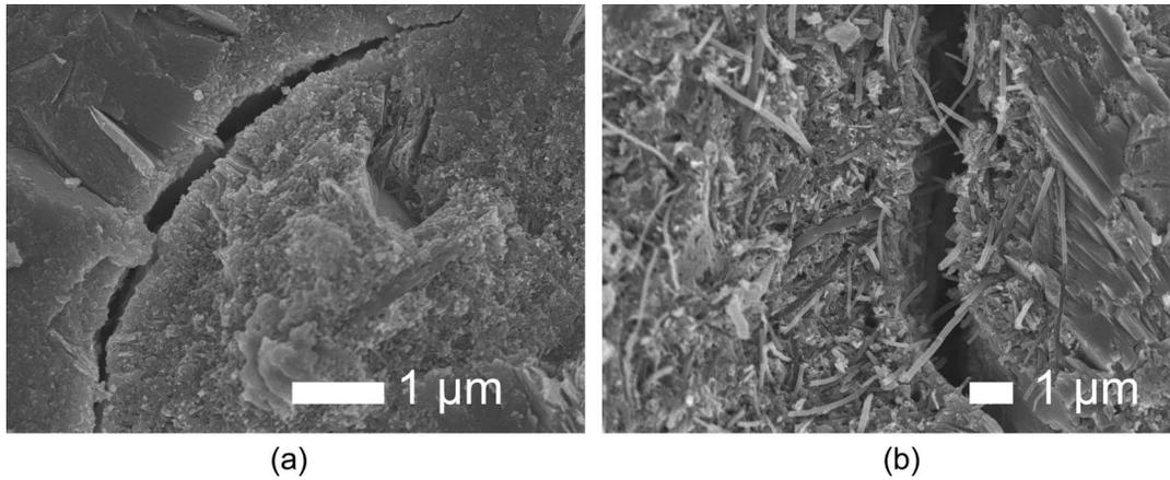
Fig. 11. (a) SEM image of the fractured surface with no CNFs within the region; (b) CNF bundled within a small area
