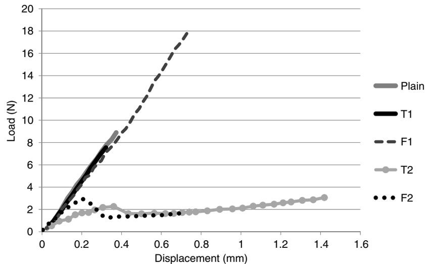
**Fig. 8.** Example of load-displacement response for the highest strength of each sample for the 7 day test
