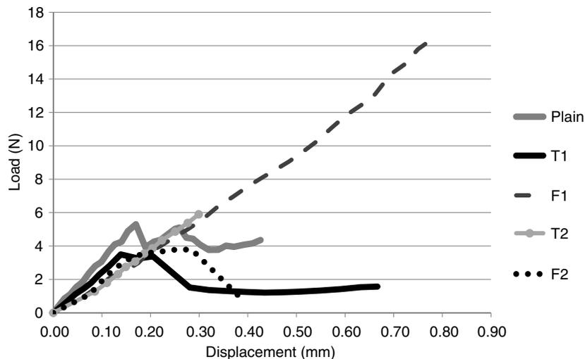
**Fig. 9.** Example of load-displacement response for the highest strength of each sample for the 14 day test
