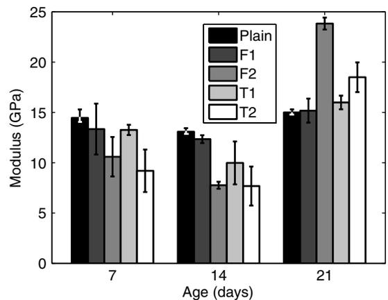
**Fig. 6.** Effect of the CNFs and MWCNTs on the elastic modulus of cement paste
