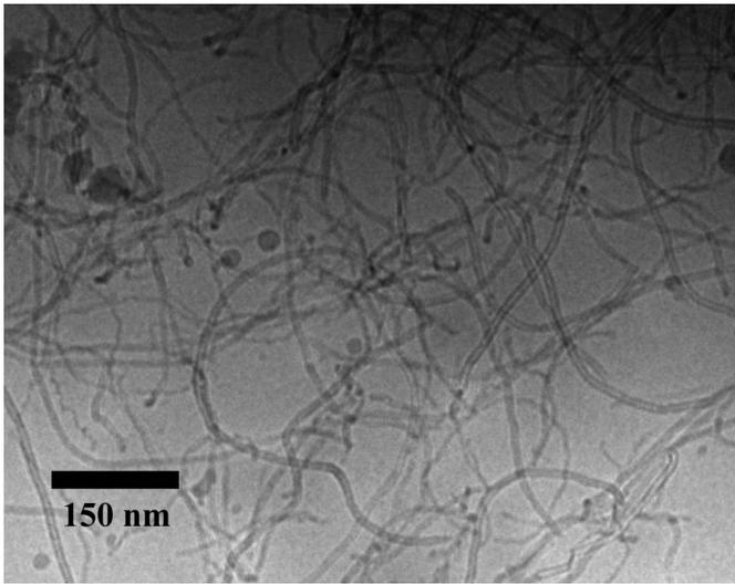
**Fig. 3.** Cryo-TEM image of CNTs dispersed in an aqueous solution; the small dark circles indicate the presence of impurities within the solution; many of the CNTs look to be intact, indicating ultrasonic mixing did not adversely affect the CNTs
