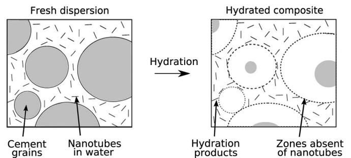
Fig. 12. Effect of cement grains on dispersibility of CNTs/CNFs; the large grains create zones that are absent of nanotubes/nanofibers even after hydration has progressed
