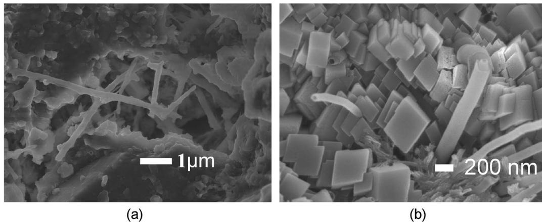
**Fig. 14.** (a) SEM image of treated CNFs embedded within the cement paste; (b) fractured end of a CNF protruding from the fractured surface of the cement
