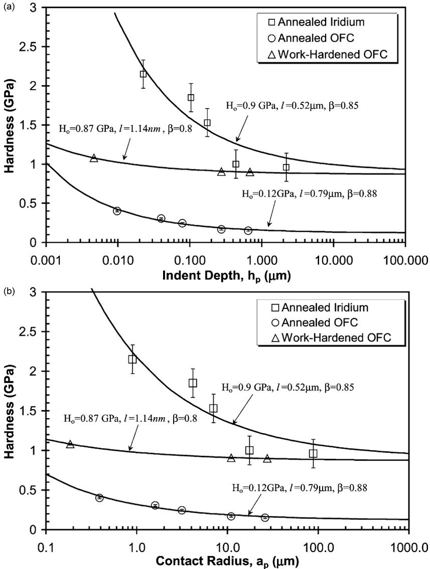
Fig. 5. Indentation size effect in iridium and oxygen-free copper measured with spherical indenters (Lim et al., 1998; Lim and Chaudhri, 1999; Swadener et al., 2002a): comparison of experiments at  $\omega = 0.025$  ( $p = 1\%$ ) with the proposed model: (a) hardness versus indentation depth [Eq. (43)]; (b) hardness versus contact radius [Eq. (33)].
