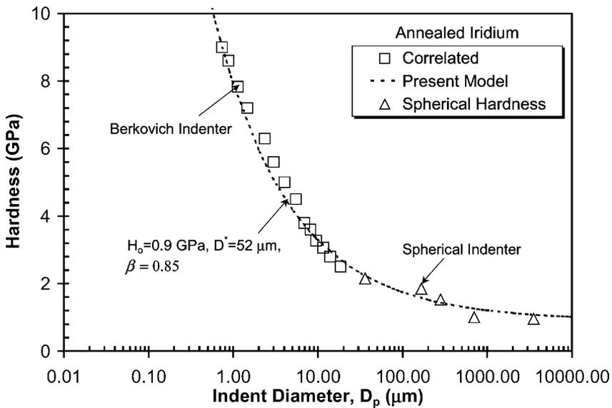
Fig. 8. Correlation of the indentation size effect in annealed irridium measured with a spherical indenter at  $\omega = 0.025$  ( $\Delta$ ), correlated from a Berkovich indenter Eq. (55) ( $\square$ ) (data from Swadener et al., 2002a), and comparison of experiments with the proposed model Eq. (37) (dotted line).
