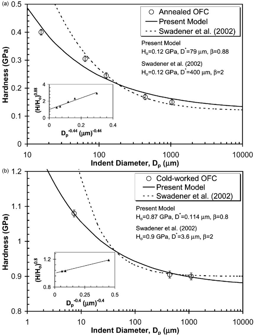
Fig. 4. Indentation size effect in oxygen-free copper (OFC) measured with spherical indenters (Lim et al., 1998; Lim and Chaudhri, 1999): comparison of experiments at  $\omega = 0.025$  ( $p = 1\%$ ) with the proposed model and Swadener et al. (2002a,b) model: (a) annealed OFC; (b) work-hardened OFC.
