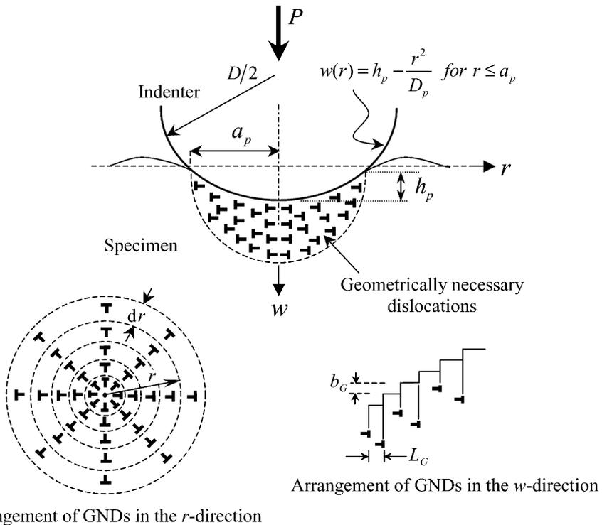
Fig. 1. Axisymmetric rigid spherical indenter. Geometrically necessary dislocations created during the indentation process. The dislocation structure is idealized as circular dislocation loops.
