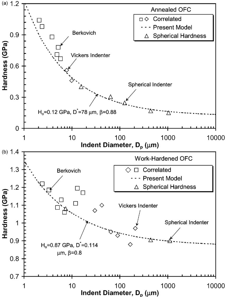
Fig. 9. Correlation of the indentation size effect in oxygen-free copper (OFC) measured with a spherical indenter at  $\omega = 0.025$  ( $\Delta$ ), correlated from Vickers ( $\diamond$ ) and Berkovich ( $\square$ ) indenters Eq. (55) (data from Lim et al., 1998; Lim and Chaudhri, 1999), and comparison of experiments with the present model Eq. (37) (dotted line): (a) annealed OFC; (b) cold-worked OFC.
