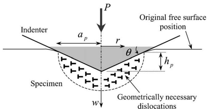
Fig. 2. Axisymmetric rigid conical indenter. Geometrically necessary dislocations created during the indentation process.
