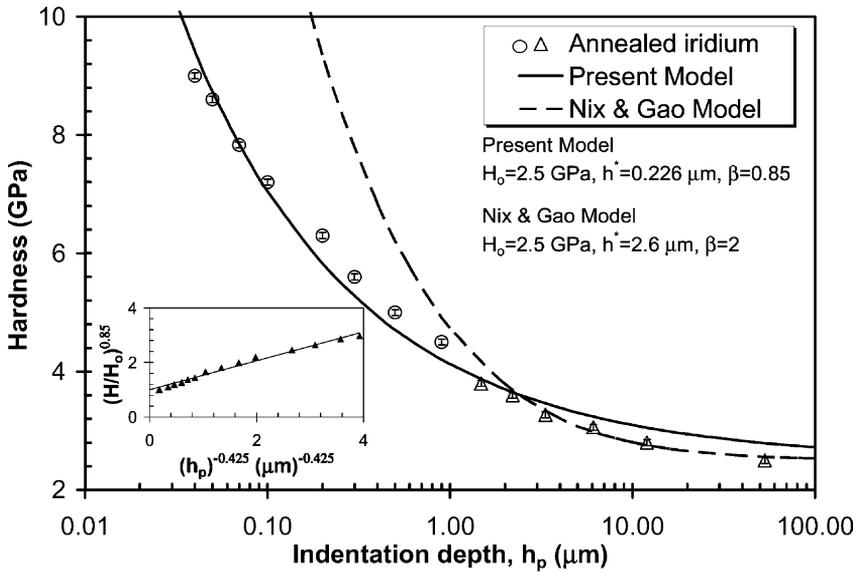
Fig. 6. Indentation size effect in annealed iridium measured with a Berkovich indenter (Swadener et al., 2002a) and comparison of experiments with the proposed model and Nix and Gao (1998) model.  $\Delta$  and  $\circ$  designate microhardness and nanohardness data, respectively.
