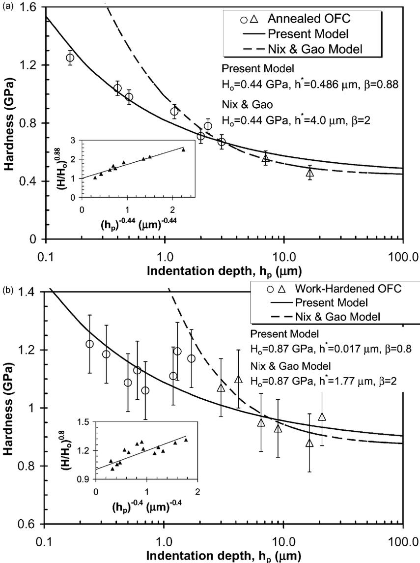
Fig. 7. Indentation size effect in oxygen free copper (OFC) measured with (Δ) Vickers and (○) Berkovich indenters (Lim et al., 1998; Lim and Chaudhri, 1999) and comparison of experiments with the proposed model and Nix and Gao (1998) model: (a) annealed OFC; (b) work-hardened OFC.
