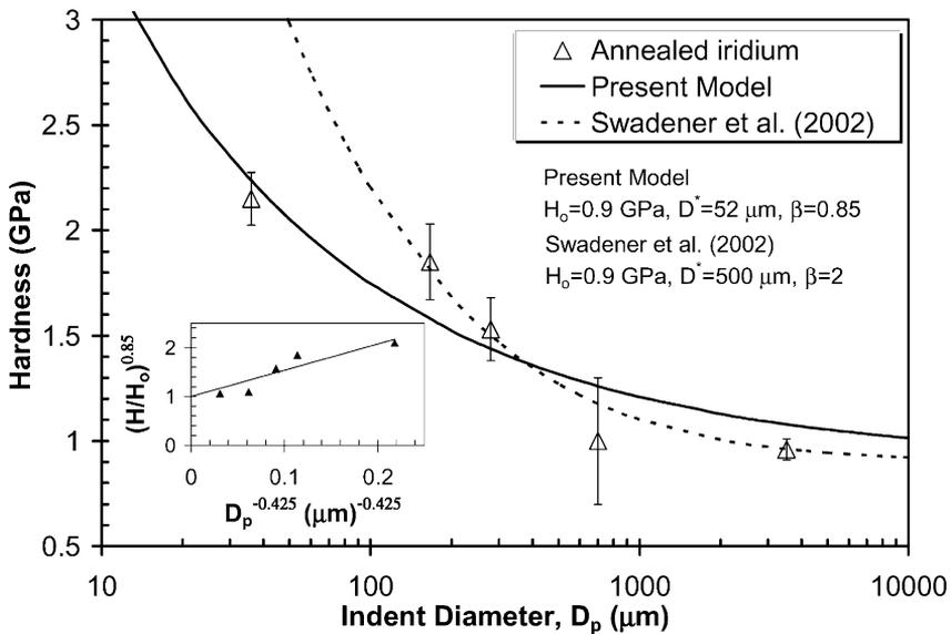
Fig. 3. Indentation size effect in annealed iridium measured with spherical indenters (Swadener et al., 2002a): comparison of experiments at  $\omega = 0.025$  ( $p = 1\%$ ) with the proposed model and Swadener et al.'s model.
