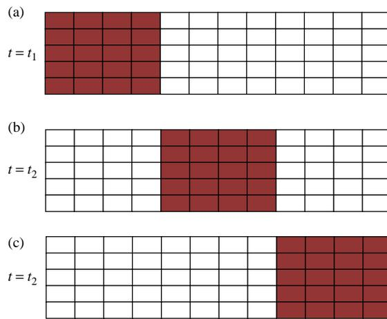
Figure 4. A schematic of the simplified wheel moving loading scenario. The shaded area is the region at which the wheel load is applied over a set of elements and then moved in the traffic direction to a new set of elements.
