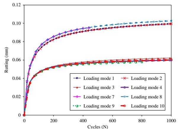
Figure 8. The rutting results for 2D plane strain and axisymmetric and their corresponding 3D FE simulations at temperature 20°C assuming an elasto-viscoplastic material constitutive behaviour.
