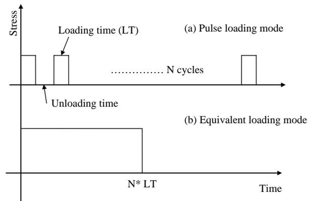
Figure 3. The sketch of equivalent and pulse loading modes. Equivalent loading is obtained by substituting pulse loading by a one step equivalent loading whose duration is equal to the summation of loading times in pulse loading.
