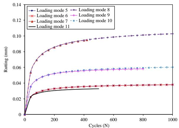
Figure 13. The rutting simulation results from 3D FE analysis at temperature 20°C assuming an elasto-viscoplastic material constitutive behaviour.
