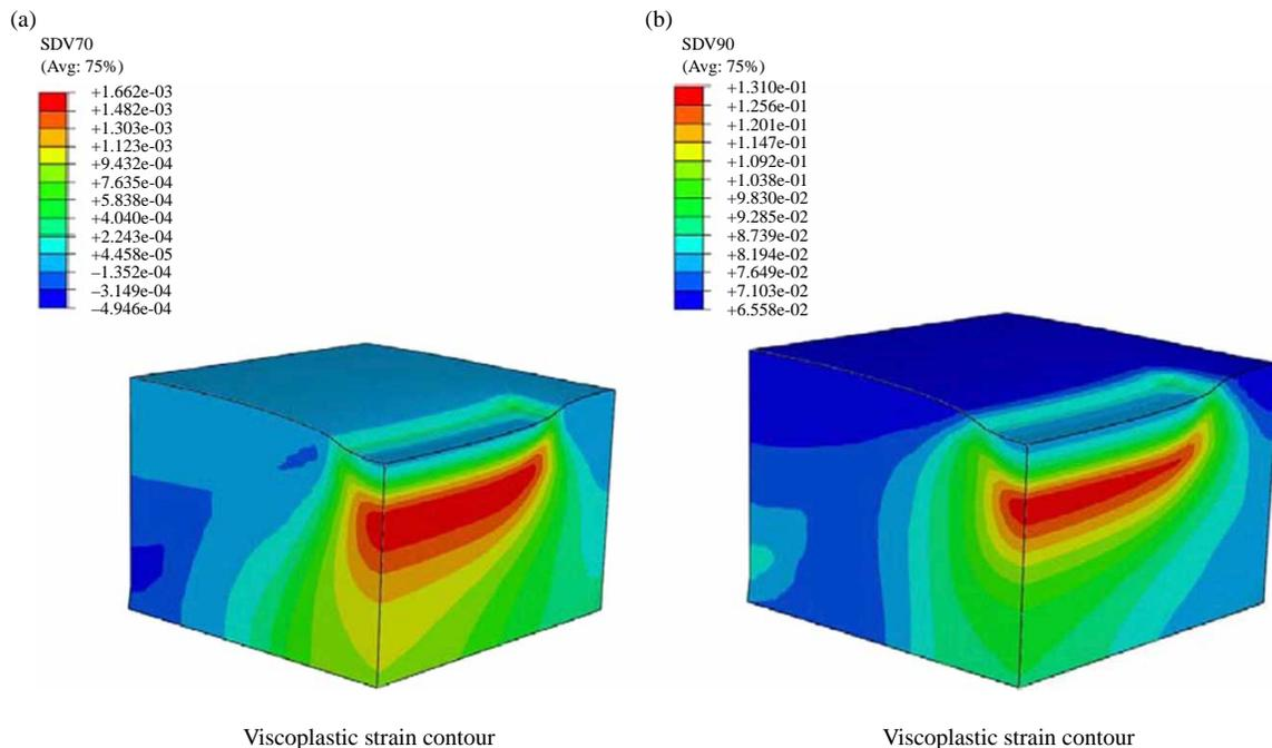
Figure 17. Viscoplastic strain and damage density distribution contours after 600 loading cycles for the 3D FE analysis when using the coupled viscoelastic, viscoplastic, viscodamage constitutive model at  $T = 20^{\circ}\text{C}$  when the pulse loading scenario is used (loading Mode 7).
