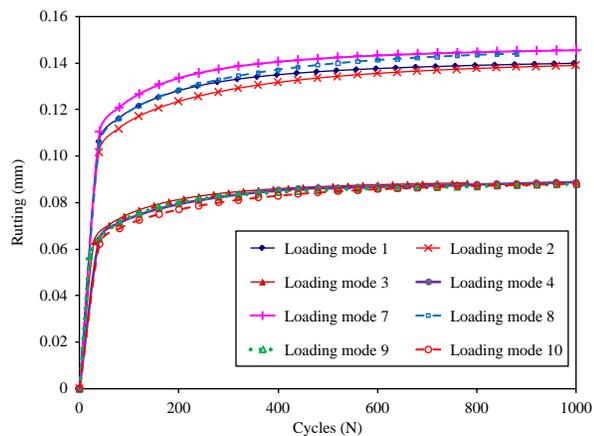
Figure 7. The rutting results for 2D plane strain and axisymmetric and their corresponding 3D FE simulations at temperature 40°C assuming a nonlinear viscoelastic and viscoplastic material constitutive behaviour.
