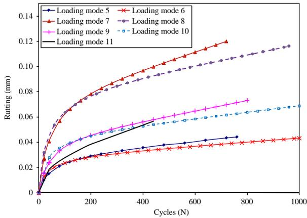
Figure 14. The rutting simulation from 3D FE analysis at temperature 20°C using the coupled viscoelastic–viscoplastic–viscodamage material constitutive model.
