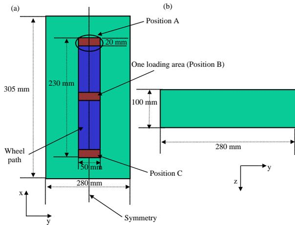
Figure 1. The geometry of the wheel tracking test. The wheel path is shown in blue, whereas the positions at which the rutting value is measured are shown in brown. (a)  $X - Y$  plane and (b)  $Y - Z$  plane.
