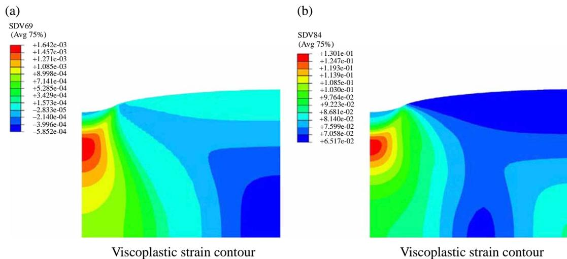
Figure 10. Viscoplastic strain and damage density distribution contours after 600 loading cycles for the 2D FE analysis when using the coupled viscoelastic, viscoplastic, viscodamage constitutive model at  $T = 20^{\circ}\text{C}$ , when the pulse loading scenario is used (loading Mode 1).
