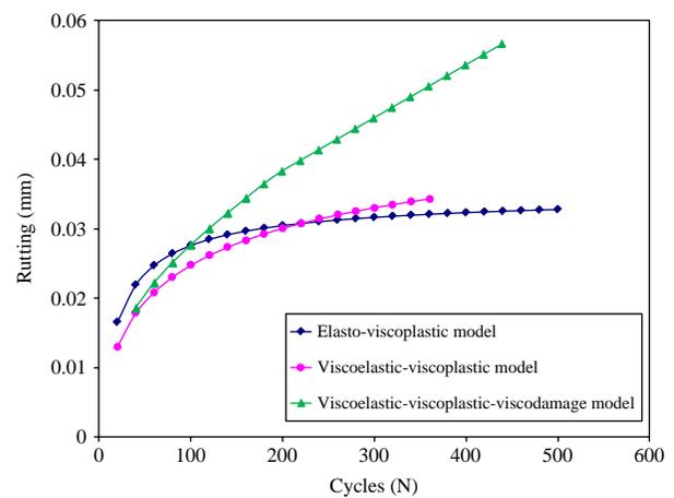
Figure 16. Comparing the rutting predictions from the 3D FE simulations using different constitutive models at temperature 20°C for loading Mode 11.
