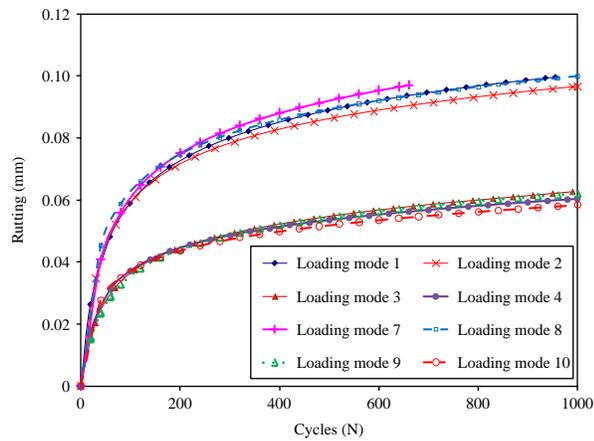
Figure 6. The rutting results for 2D plane strain and axisymmetric and their corresponding 3D FE simulations at temperature 20°C assuming a nonlinear viscoelastic and viscoplastic material constitutive behaviour.
