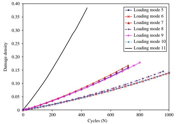
Figure 15. The evolution of the damage density from 3D FE analysis at temperature 20°C using the coupled viscoelastic–viscoplastic–viscodamage material constitutive model.
