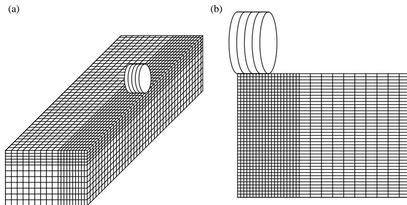
Figure 2. The FE mesh in (a) the 3D simulations and (b) the 2D simulations.
