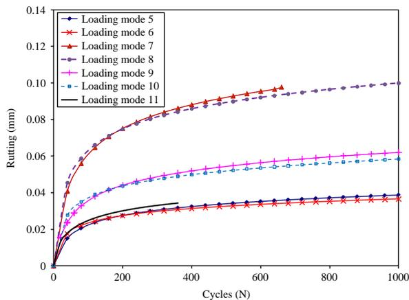
Figure 11. The rutting simulation results from 3D FE analysis at temperature 20°C assuming a nonlinear viscoelastic and viscoplastic material constitutive behaviour.
