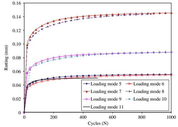
Figure 12. The rutting simulation results from 3D FE analysis at temperature 40°C assuming a nonlinear viscoelastic and viscoplastic material constitutive behaviour.
