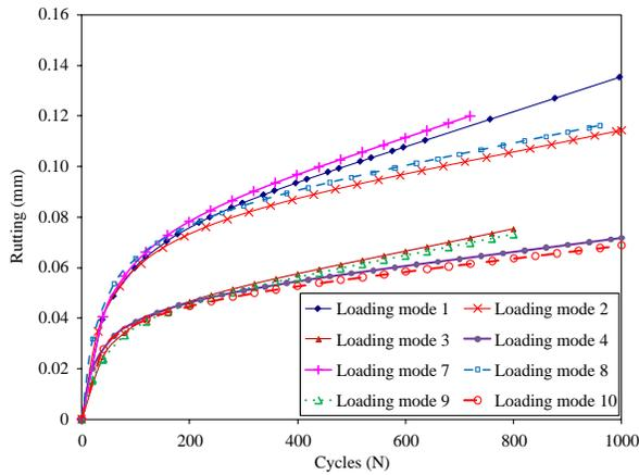
Figure 9. The rutting results for 2D plane strain and axisymmetric and their corresponding 3D FE simulations at temperature 20°C using the coupled viscoelastic–viscoplastic–viscodamage material constitutive model.
